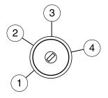
the 4 (start) position, the engine may continue cranking for up to 10 seconds or until the vehicle starts.
